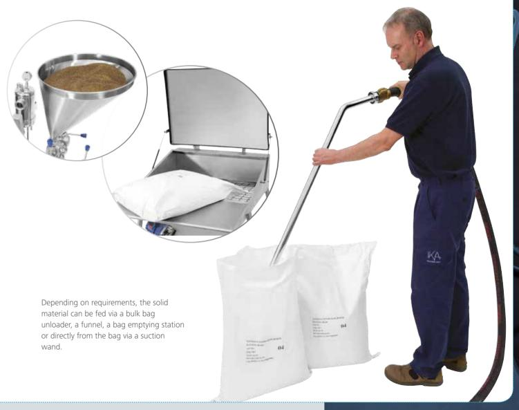
The CMX is commonly used in a recirculation process. An appropriate quantity of solids is incorporated into a fixed volume of liquid using the inline device. The CMX offers a simple, functional and cost-efficient method of incorporating solids into liquids, without the need for additional powder dosing systems or pumps. In a highly efficient inline process, small volumes of powder are dispersed into a highly turbulent area free of agglomerates.
