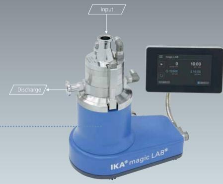
The DR/DRS is a high-shear dispersing machine for the production of microemulsions and ultra-fine suspensions, for wet milling and for dissolving processes. Whilst the production machines of type DR are operated with standard circumferential speeds of approx. 23 m/s and 3 tools, with the magic LAB®, the fast-running variant of type DRS with circumferential speeds of up to 40 m/s and 2 tools in series can also be simulated.
