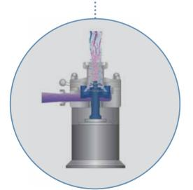
Corundum disk mills are for the ultra-fine milling of granules and tough pastes and for the wet milling of viscous products or fruits with a high liquid content.
