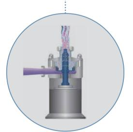
The UTL is a single-stage dispersing machine for the production of emulsions and suspensions with a coarse or medium particle size and a narrow particle size distribution. There are numerous rotor-stator variants, enabling the adaption of the machine to the respective application.
