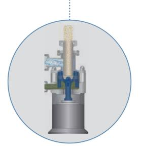
The CMS was developed for the dust-free incorporation and dispersing of powdery solids into liquids. It uses a specially developed rotor that generates a high suction force, thus sucking in the solid and incorporating it into the liquid. The liquid is circulated until all of the powder has been incorporated.
