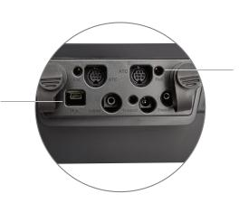
Measure pH, ion concentration (ISE), mV, relative mV or ORP with temperature using the meter's two BNC, reference pintip and ATC temperature inputs
