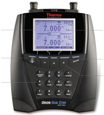
Selectable read modes include Auto-Read, On-Ready, At Timed Intervals, Continuous, Value Change in Measurement and Timed for a variety of measurement collection methods for different analytical methods
