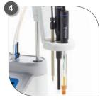
Bottle holder helps secure titrant to prevent spills and can be easily disconnected from the titrator for flexible placement on the lab bench.
