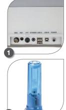
Titrator connections have clearly labeled functions, including three USB ports for printer, USB flash drive, and computer software connections.
